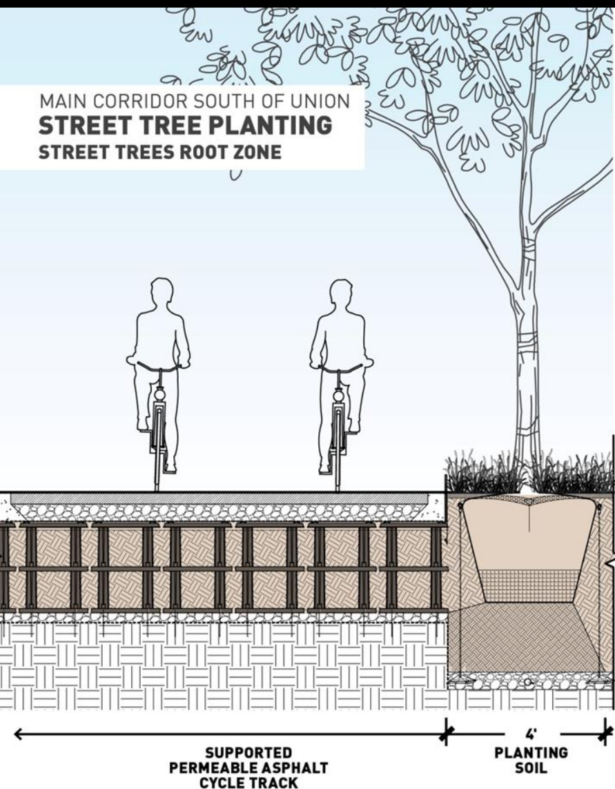
WEST-SIDE SOIL CELLS UNDER CYCLE TRACK
